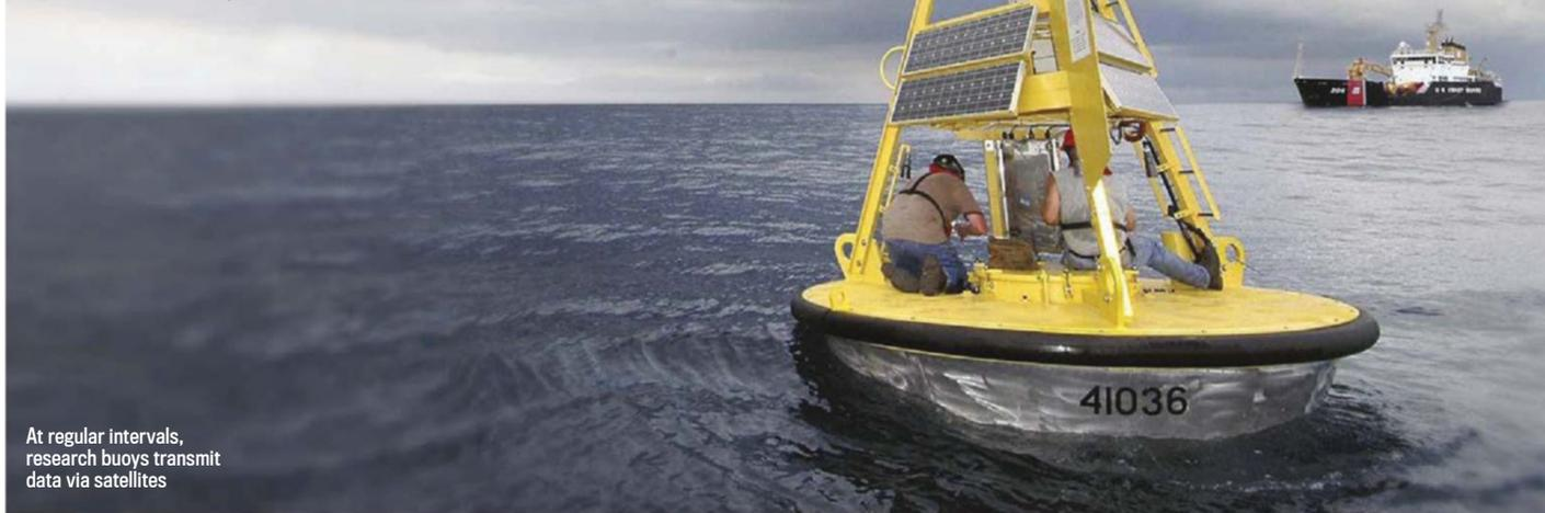
At regular intervals, research buoys transmit data via satellites
