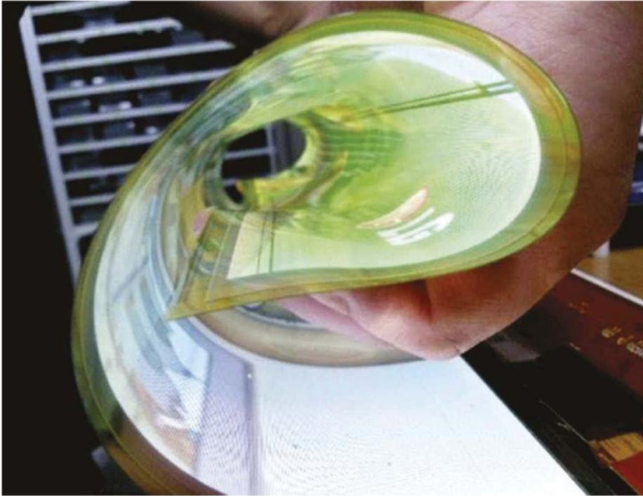
OLED screens can be mounted on a flexible plastic substrate, enabling them to be rolled up when not in use
